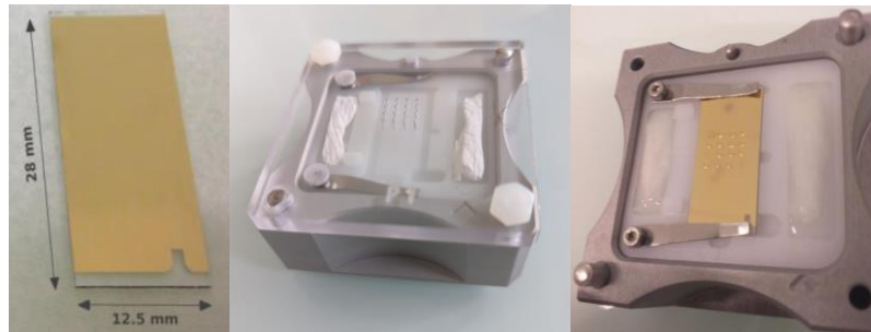
Figure 2: Gold biochip (left), micropipette spotter (middle) and the biochip after spotting with ligands droplets of 300 nl each (right).
