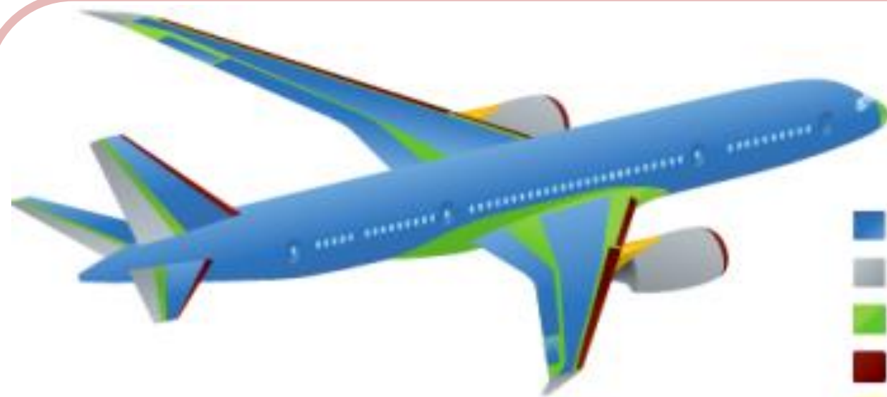
Boeing 787 Dreamliner Composite Components
