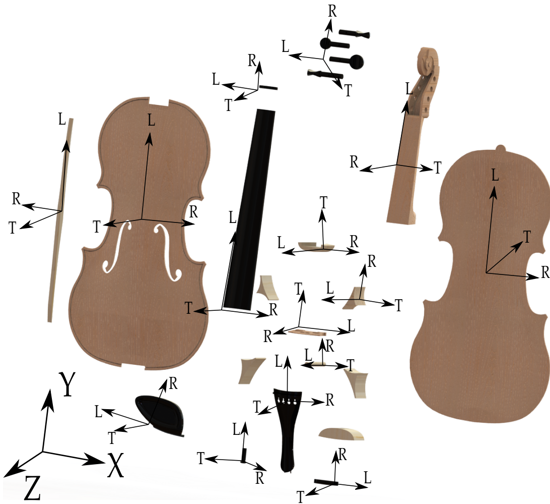
Figure 6: Scheme of the material orientation of the parts in the violin.
