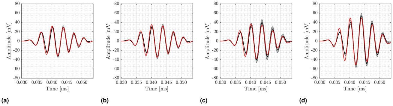
**Figure 13.** Model response for PZT at (a) 0 °C; (b) 10°C; (c) 30°C; and (d) 60°C. In the graphs, the colors represent experimental 50 mm damaged signal (—), model prediction for 50 mm with mean properties (—) and confidence interval (■).
