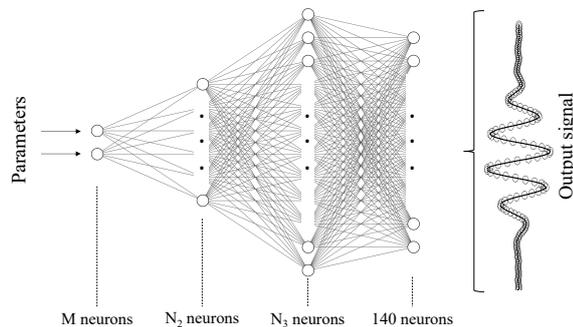
**Figure 9.** Architecture of the MLP used as surrogate-model.
