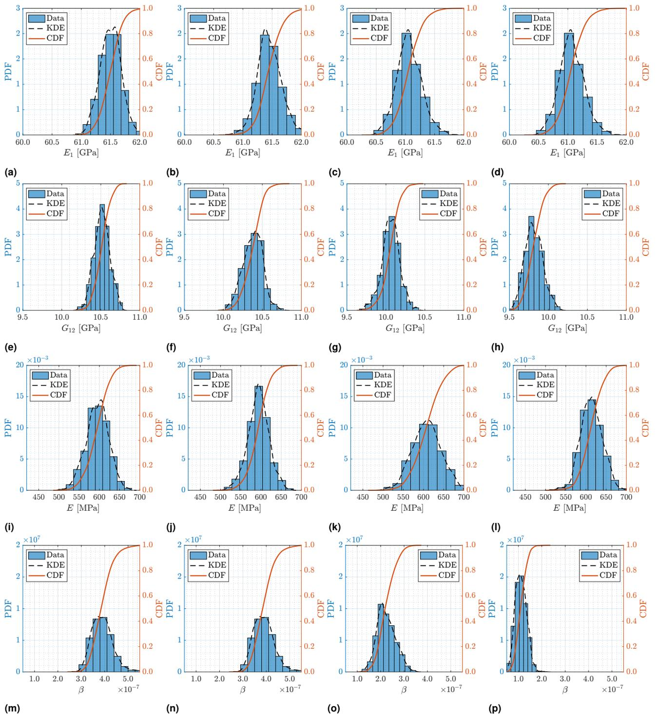
**Figure 12.** Results for stochastic updating procedure using 30, 50, and 70 mm damage diameters at 0, 10, 30, and 60°C, respectively, in the horizontal direction. (a) to (d)  $E_1$  distribution; (e) to (h)  $G_{12}$  distribution; (i) to (l)  $E$  distribution; and (m) to (p)  $\beta$  distribution. In the histograms, the colors represent: Sampled data (■), Kernel Density Estimate (KDE) (---) and Cumulative Density Function (CDF) (—).
