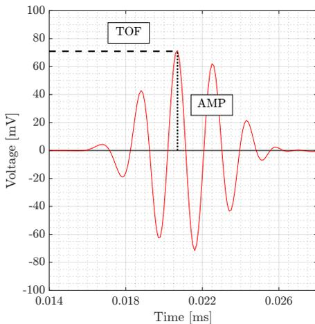
**Figure 3.** Metrics used at sensitivity analysis
