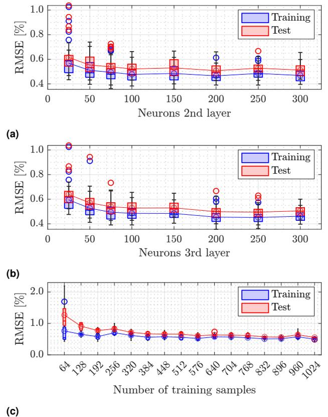
**Figure 11.** Surrogate model RMSE in training and test data with respect to: (a) number of neurons in the second layer; (b) number of neurons in the third layer; and (c) samples used in the training phase.
