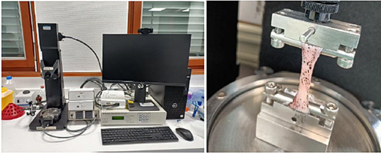
FIGURE 3 Test machine Mach-1® (Biomomentum Inc, Canada) and grips for soft tissues.
