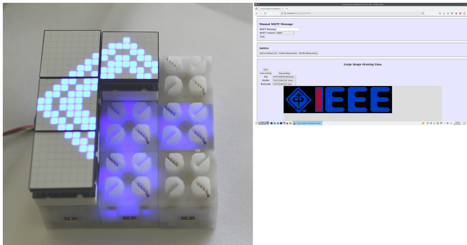
Fig. 4: The setup made of 4 D-XBlocks and 5 Blinky Blocks building a part of our multi-resolution display. The bottom image is a screenshot of the web control interface on the Wi-Fi-connected master computer.
