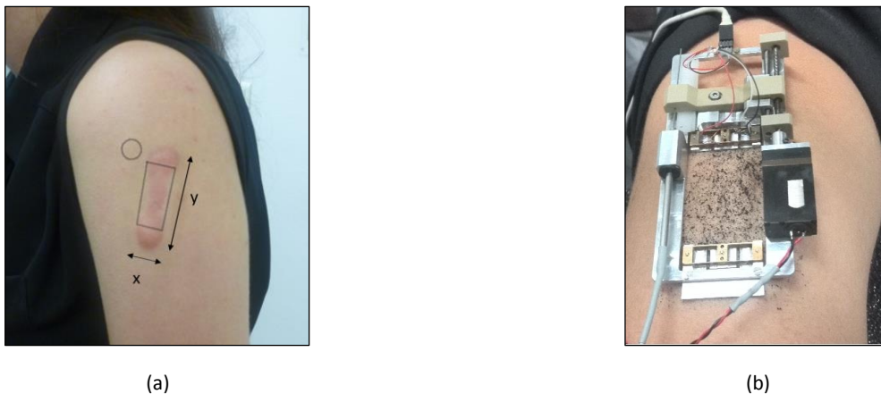
Figure 1. Experimental investigation into the mechanical response of keloid scar (from Chambert et al. 2019 [2]). (a) Butterfly-shaped keloid ( x=15\text{mm} , y=47\text{mm} ). (b) A uni-axial was test carried out on a butterfly-shaped keloid with an extensometer.
