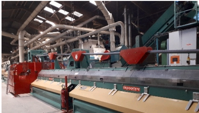
Fig. 2. Industrial scutching/hackling extraction device available at Terre de Lin.
