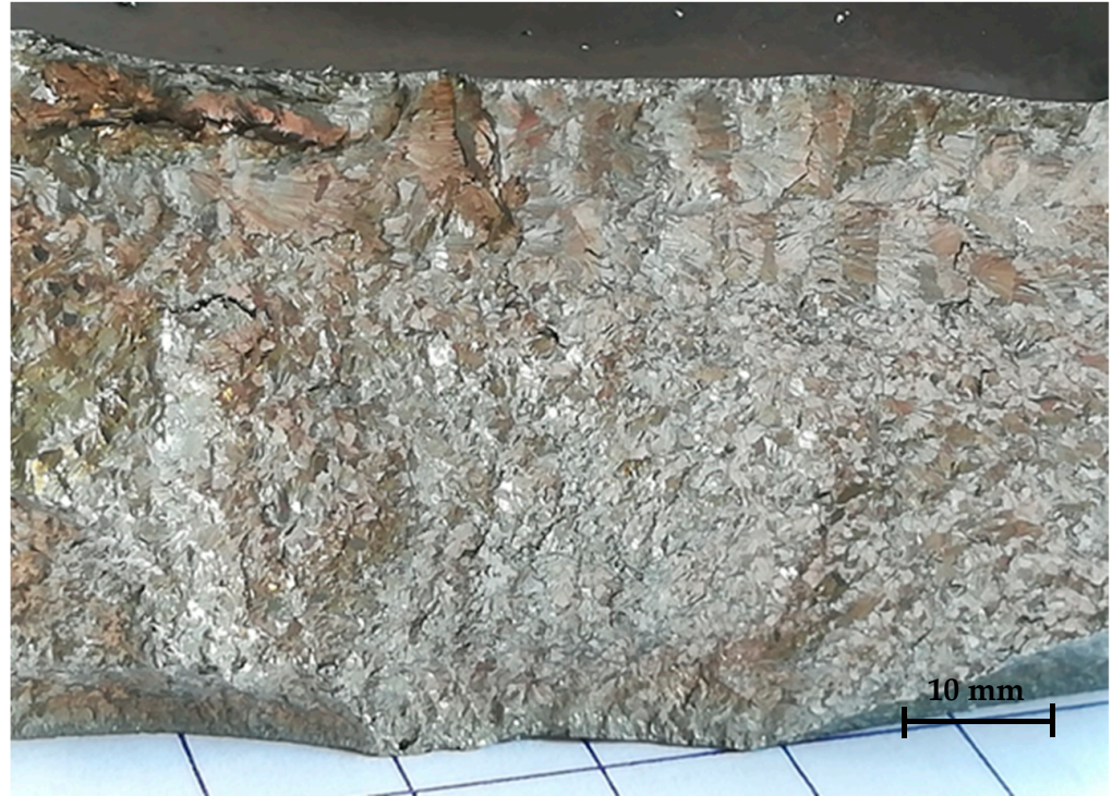
Figure 2. Surface generated by brittle fracture of a 40 mm thick rectangular \text{Ti}_{0.5}\text{Fe}_{0.45}\text{Mn}_{0.05} ingot. The lower surface was in contact with the copper mold, while the upper surface was a free surface.
