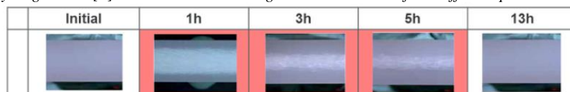
Figure 1: Cross section of HDPE monolayer liner before and after depressurization (from 87.5 MPa to 2MPa in 1, 3, 5, and 13 h depressurizations at 50 °C) observed by tomography [3]
