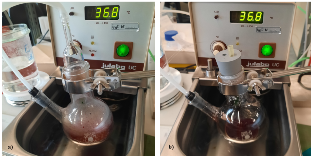
Fig. 19. Blood deoxygenation setup. a) deoxygenation with output gas tubing. b) Output gas tubing is removed and replaced with the rubber stopper. The single core TPU probe fits through it.
