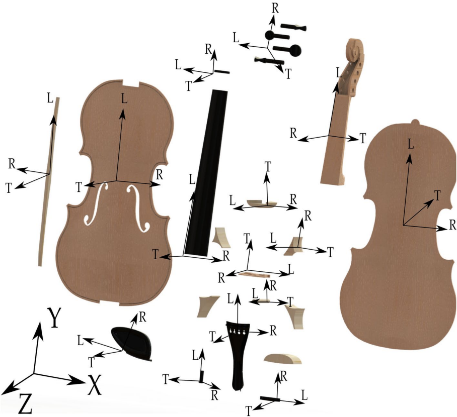
Fig. 9. Scheme of the material orientation of the parts in the violin.
