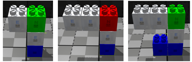
Fig. 7: Three Experiments on VisibleSim , the Head Block is Green if the Structure is Balanced and Red Otherwise.
