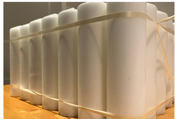
FIG. 6. Photograph of an experimental realization of a two-dimensional phononic crystal structure, consisting of a 7 \times 7 array of touching paraffin wax candles with radius R = 4 \text{ cm} .
