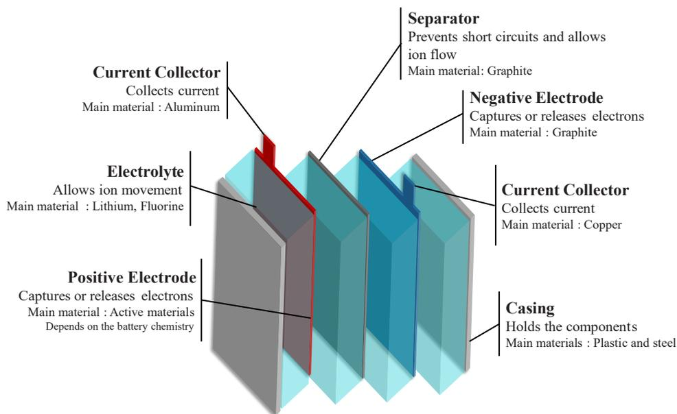
**Fig. 3.** Schematic representation of a lithium-ion battery cell, showing the main components and their primary materials. These materials vary depending on the specific battery chemistry.
