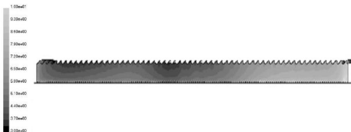
Figure 7. Carbon dioxide dispersion in a 60 span Venlo-type glasshouse with crops (Reichrath and Davies, 2001).
