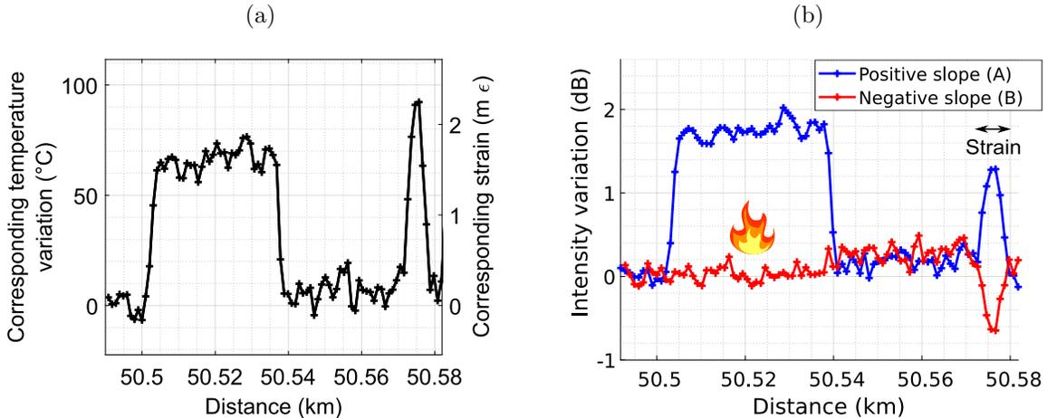
Figure 4: (a) Conversion of the frequency shift into an equivalent temperature variation and strain from measurement shown in Fig. 3. (b) Identification of strain and temperature effects, with a comparison between the intensity variation measured on operating point A (positive slope) with operating point B (negative slope). Measurement realized with the  $\nu$ -BOTDR with a 2 m spatial resolution, and a 1 m sampling interval.
