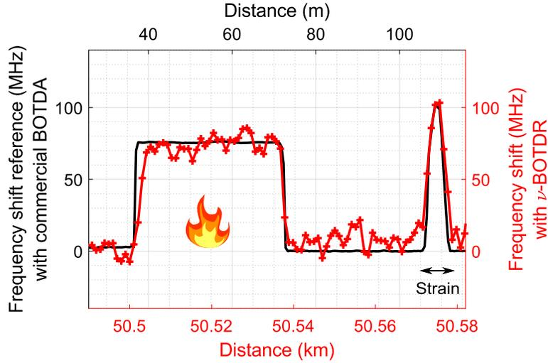
Figure 3: Comparison between the reference frequency profile get with a commercial BOTDA (Ditest, Omnisens) realized at 50 m in black, and a measurement of the frequency profile measured with the  $\nu$ -BOTDR at 50 km, in red. Both measurements were obtained with a spatial resolution of 2 m.
