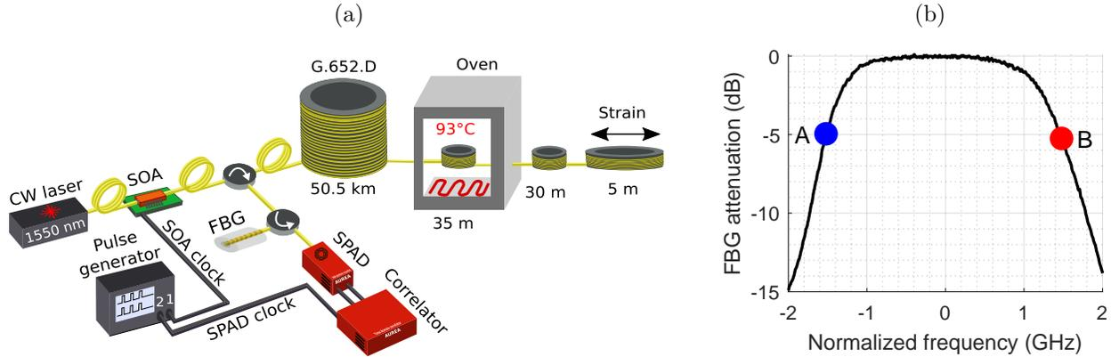
Figure 2: (a)  $\nu$ -BOTDR experimental setup, with an experimental bench of temperature and strain measurements. (b) Fiber Bragg grating (FBG) response, with the operating points A and B.
