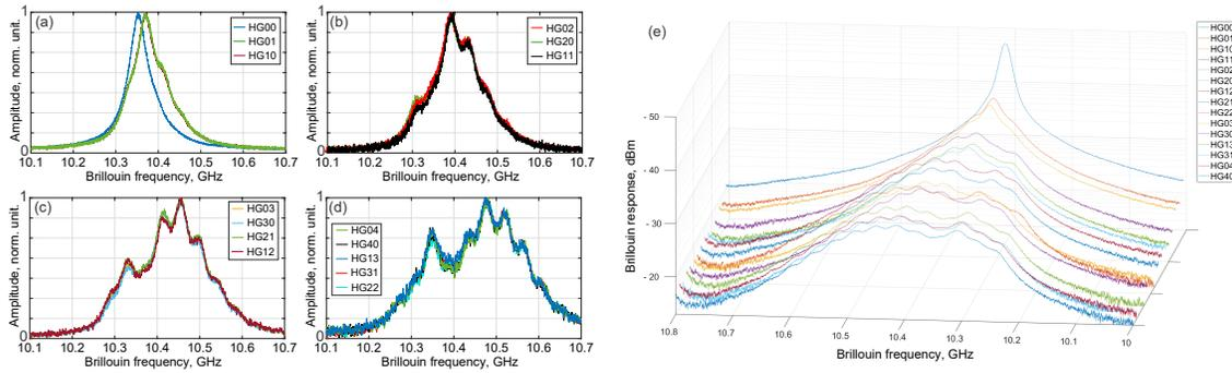
Figure 2. Spontaneous Brillouin measurement obtain with heterodyne detection and Multiplexer for injection in different optical mode. (a) normalized Brillouin spectrum for the different family of optical mode. (b) Waterfall of spontaneous Brillouin spectrum for the same input power. The Brillouin efficiency decrease when the number of spatial mode increases.
