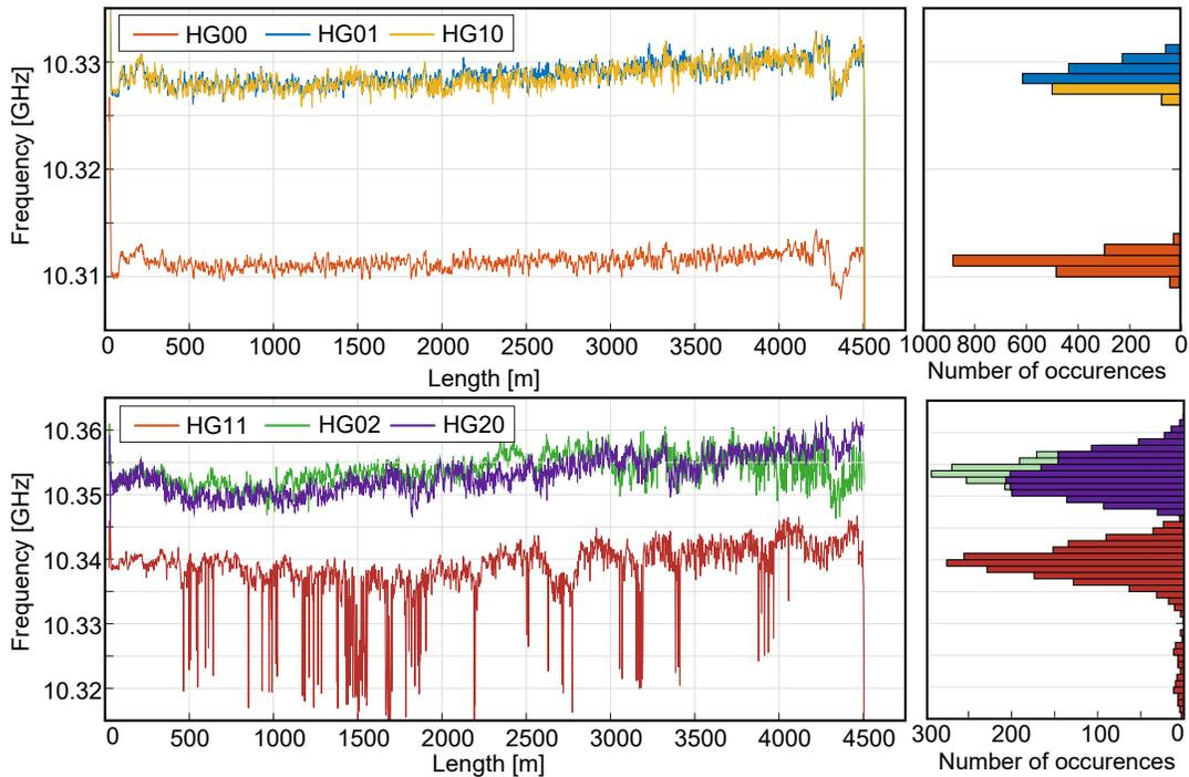
Figure 3. Distributed Brillouin frequency recorded with the Ditest instrument all along the graded index multimode fiber for injection in the first six different optical modes. The experimental parameter were : frequency step 1 MHz, sampling 2.5 m, spatial resolution 10 m, 5000 average. At the right, integrated Brillouin frequency calculation for the different tested optical modes.
