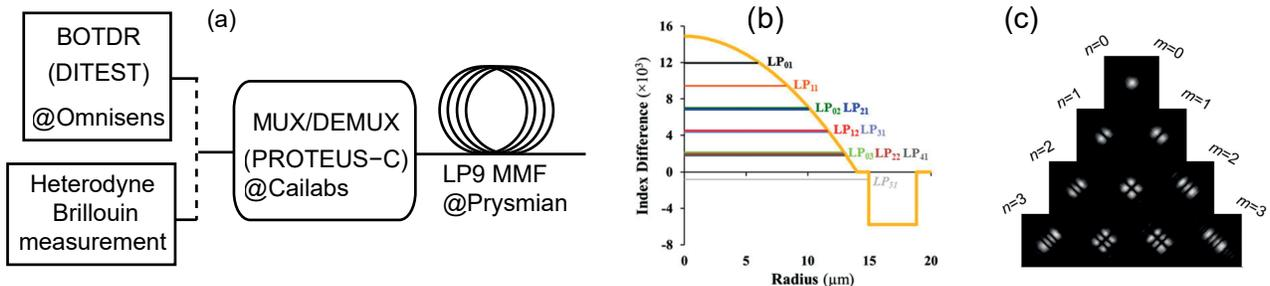
Figure 1. (a) Experimental setup. The length of optical fiber is 4.5 km. (b) Refractive index profile of LP9 multimode optical fiber from reference.<sup>4</sup> (c) Theoretical representation of optical spatial mode from cailabs.com.
