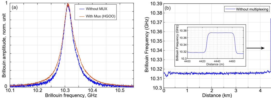
Figure 4. (a) Spontaneous Brillouin spectrum measurement with heterodyne detection along the 4.5 km of graded LP9 fiber direct measurement (blue) and injection on HG00 optical mode with multiplexer. (b) BOTDR measurement with DITEST in LP9 without multiplexing. A hot spot of 30 m with a temperature of 80°C is applied at this end of the fiber with spatial resolution of 5 m.
