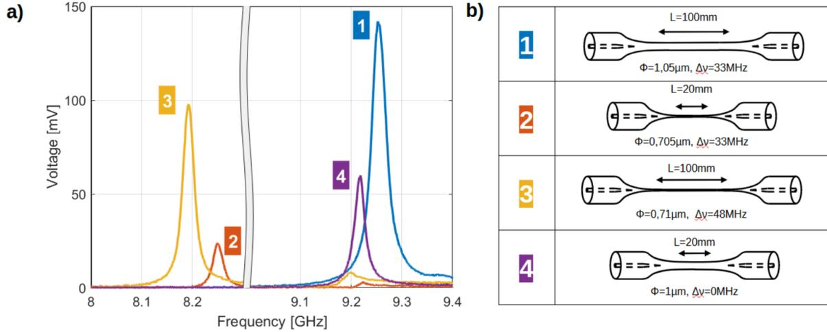
Figure 2. **Characterization of the nanofiber samples** a) Spontaneous Brillouin spectrum of the ONFs. b) ONF geometrical characteristics.
