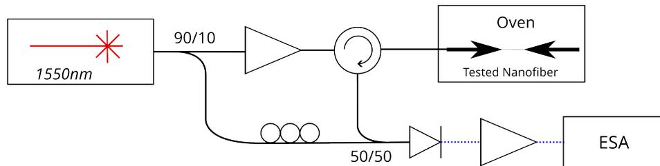
Figure 1. Experimental setup of a Brillouin heterodyne detection, with the nanofiber under test placed in a controlled temperature oven. The pump laser is a high coherent continuous fiber laser with a linewidth of 10 kHz. Blue dotted lines represents the electrical links. ESA is an electrical spectrum analyzer.
