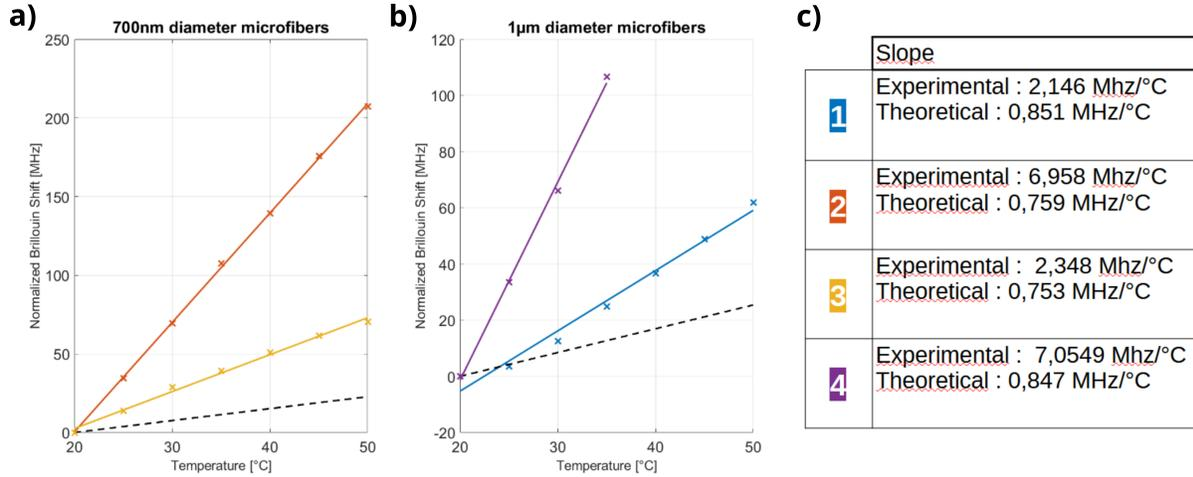
Figure 3. (a,b) Normalized Brillouin frequency shift of the ONF's, for a temperature variation range of 20°C-50°C. The dashed line represents the temperature coefficient in standard silica fiber. c) Slopes values corresponding to temperature coefficient of the ONF's. are summarized. The theoretical value are present for comparison.
