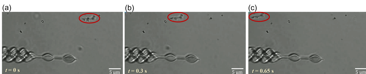
Fig. 5 | Using a laser power of 30% to achieve high translational velocity. a The OPTOBOT at the beginning of the translation. b The OPTOBOT after 0.3 s. c The OPTOBOT after moving 34 μm in 0.65 s, giving a translational velocity of 52 μm/s.
