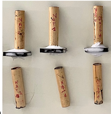
Figure 6 (a) Sample in the oven at 100°C before the pull-off test; (b) Samples after the pull-off test.
