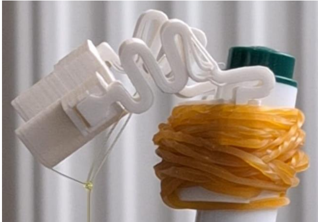
Fig. 7. Photography of the 3D-printed orthoses after failure with a weight of 700 g.
