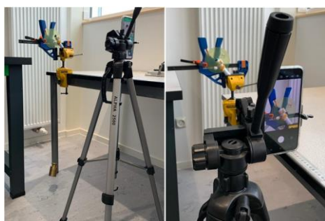
Fig. 2. Experimental set-up for angular displacement measurement for commercial orthoses. The main parts are a smartphone for image recording, a clamping system with a bench vise mounted on a swivel, a tube to fix the orthosis and a protractor.
