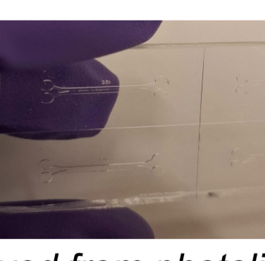
PDMS removed from photolithography mold
