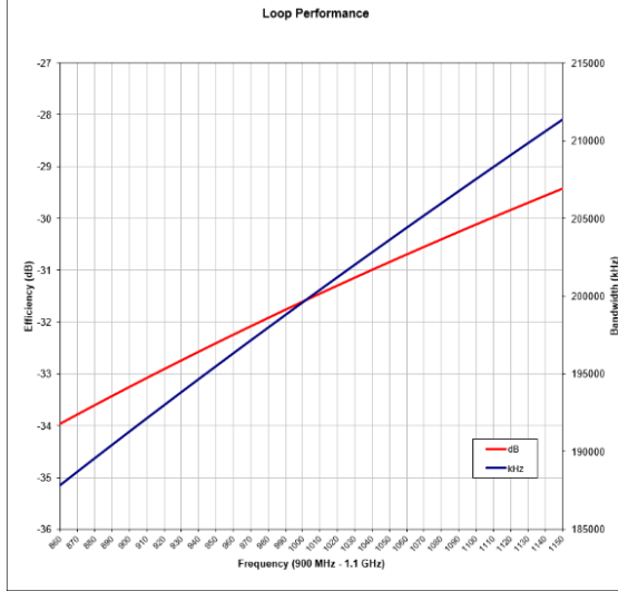
Figure 3. Efficiency (in dB) and frequency bandwidth (expressed in kHz) of the main loop antenna versus frequency expressed in MHz is determined according to the 1.01 GHz centered frequency, 9.5 mm diameter, Gold electrical parameters – see Table 2, and based on the work of. Q-factor is predicted at 5.05 and measured at 4.98.
