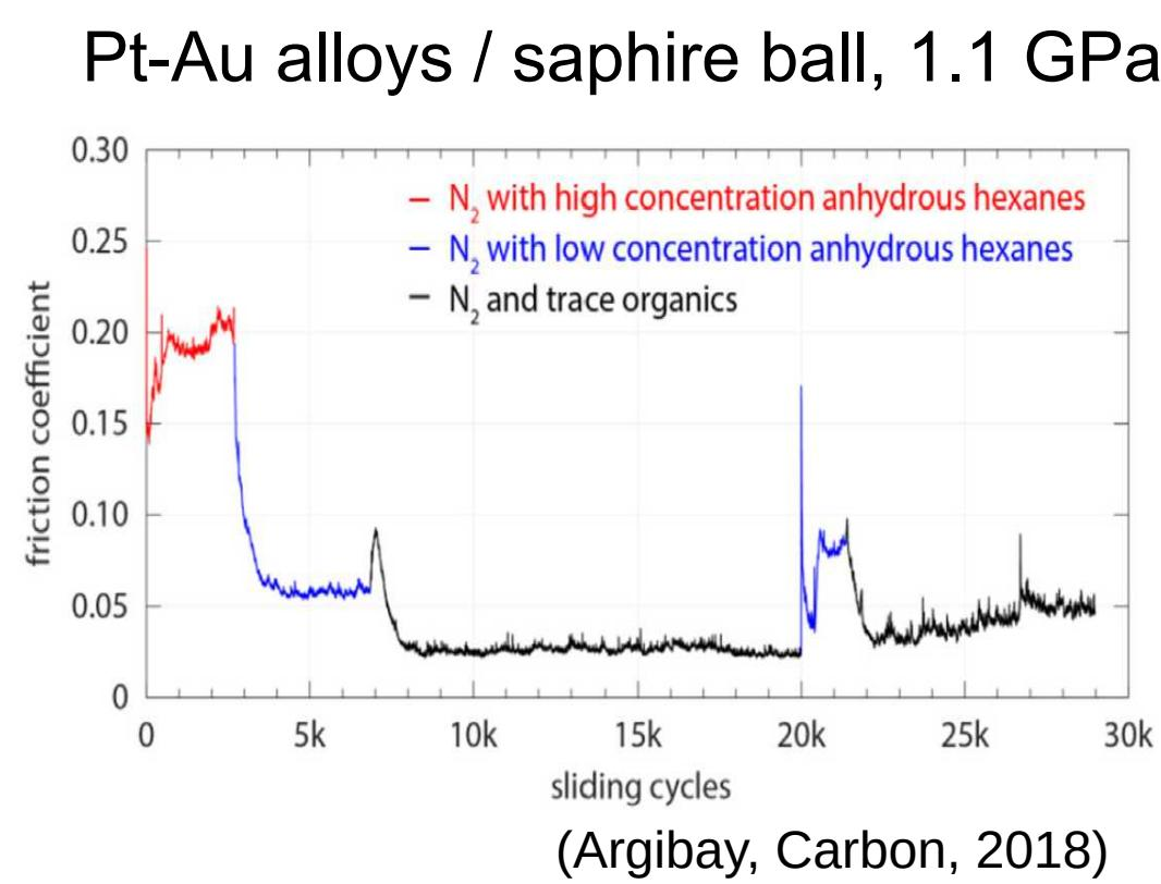
A tribofilm forms from trace airborne organics during sliding, acting as a lubricating third body
