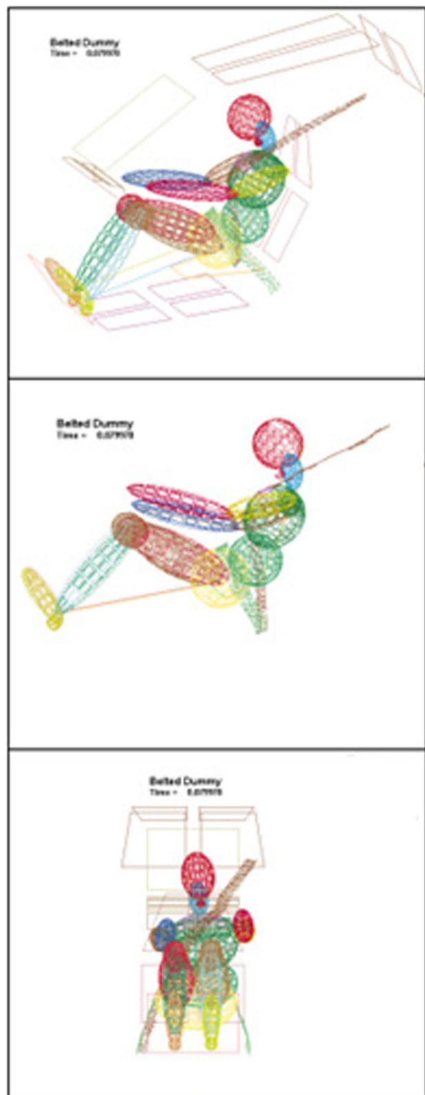
Fig. 9 Dummy response in the crash process—frontal impact at 70 km/h
