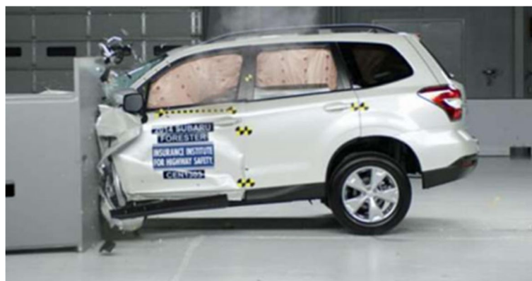
Fig. 1 Frontal crash of a vehicle at a speed around 100 km/h. Data taken from Ref. (Tabiei and Wu 2000)
