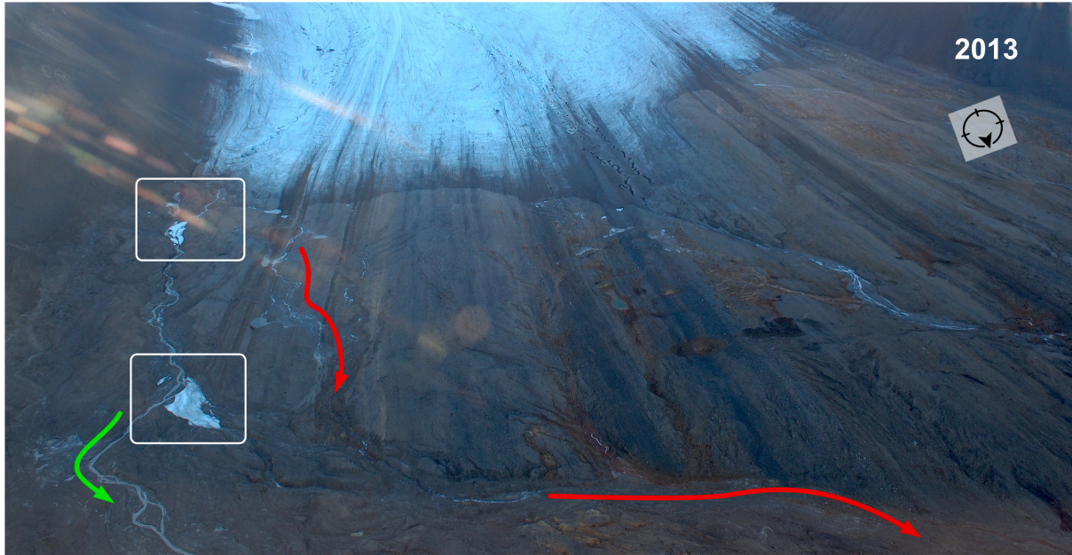
Figure 14: Opportunistic aerial image of Austre Lovénbreen collected in 2013 illustrating the impact of upstream and downstream icings (white squares) driving all water flows to the eastern outlet rather than the western outlet collecting all outgoing water streams as seen on Fig. 13. The arrows guide the eye towards active water flows (green) and inactive channels (red) with the direction of flow determined by the arrow head.
