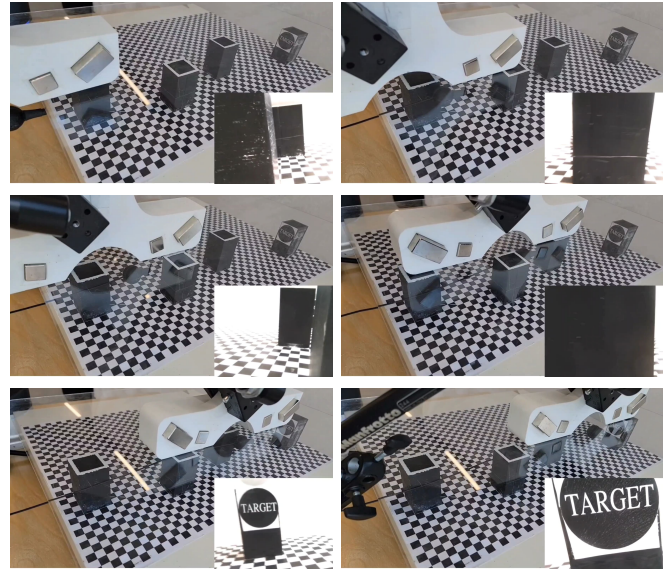
Fig. 14. Open-loop telemanipulation of the weight-compensated endoscope demonstrating obstacle avoidance from initial to target position.
