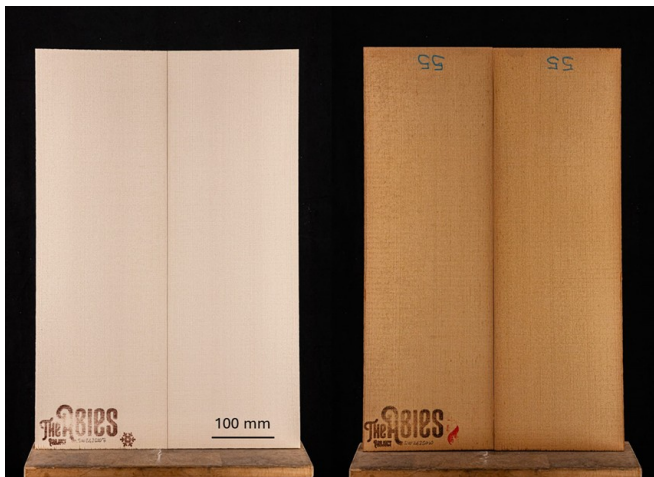
FIG. 2. An example of two different bookmatched spruce boards similar to those considered in this study in their pristine state (left) and thermal treated at 160^{\circ}\text{C} (right). Boards thickness is 5 mm. Photo Courtesy Wood 'n' Tones 22 .
