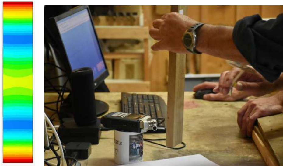
Figure 4: Measurement examples. Left: first bending mode, blue color corresponds to nodal lines, simulations made with the software Simscale (Gmbh 2024). Practical Workshop made with makers, measurement of the first bending frequency on a wood beam.
