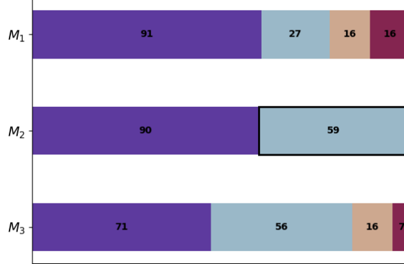
Figure 2: An optimal schedule for instance in Fig. 1. The makespan is C_{\max} = 150 . The black framed job represents an assignment on the second least loaded machine, other assignments are all made on the first available machine (wrt LS)
