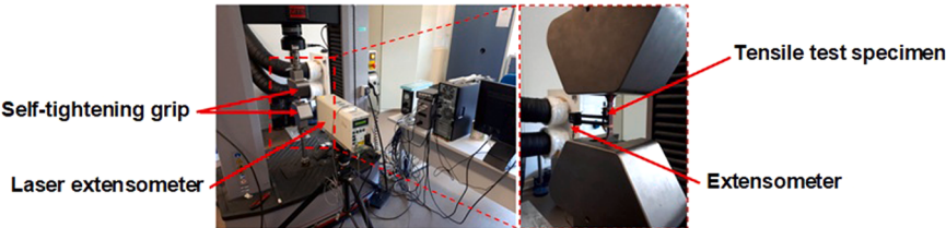
Fig. 9. A photograph of Lloyd EZ20 universal testing.
