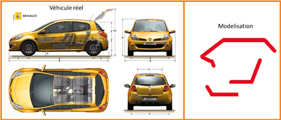
Fig. 4. Comparison between the geometry of the vehicle and its simplified 3D digital model.
