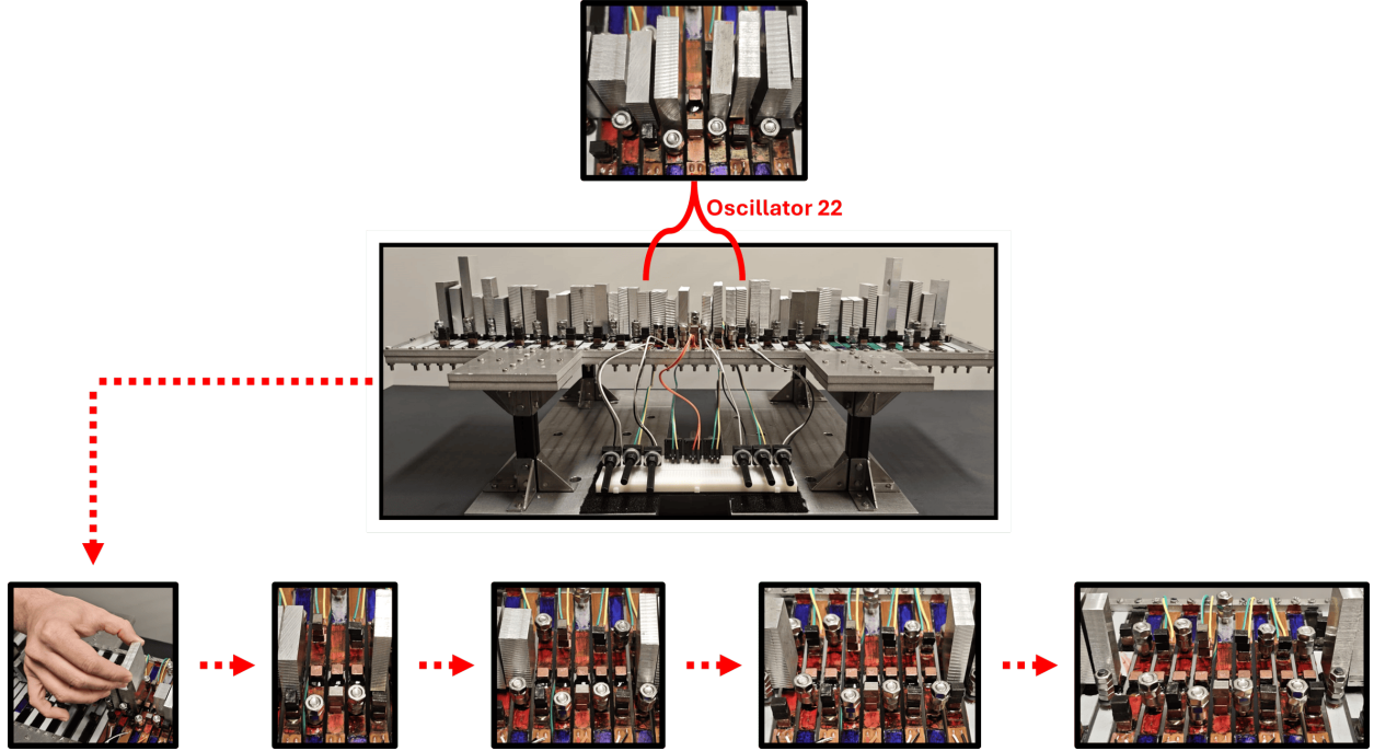
FIG. 7. Experimental strategy for studying isolated oscillators. Aluminum masses gradually allowed to oscillate, starting from the central oscillator (index 22).
