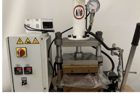
(a) Hot press used for the manufacturing of the composite plates.
