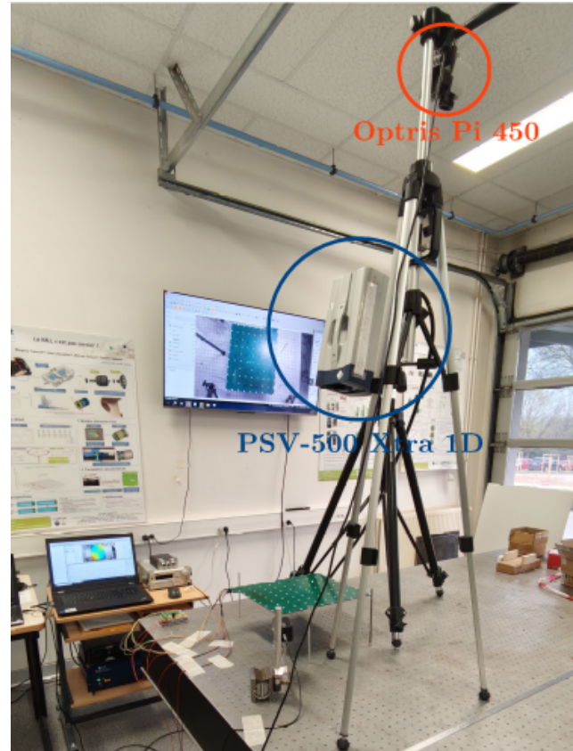
(b) Instrumentation: PSV-500 Xtra 1D laser vibrometer and Optris PI 450 thermal camera.
