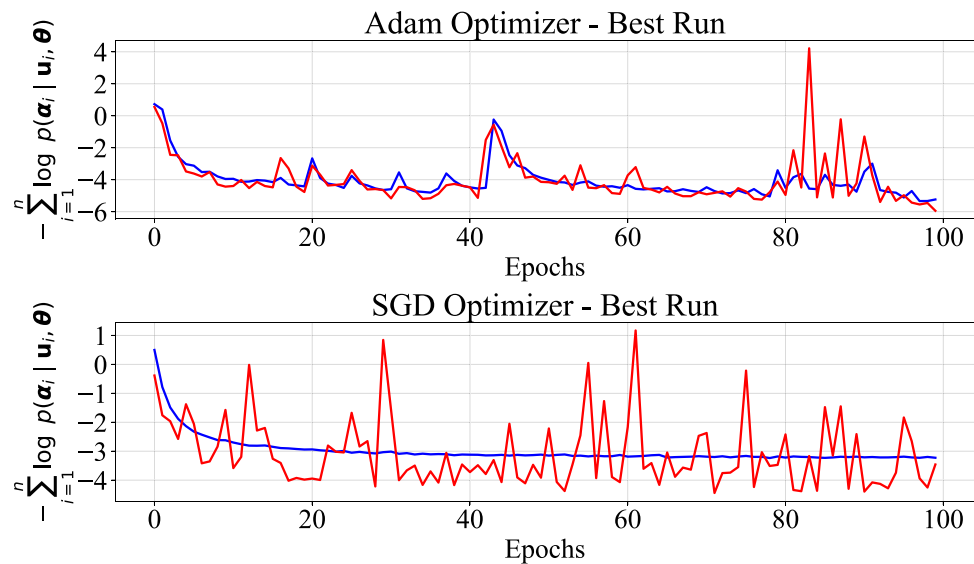
Fig. 6 Best training runs of the BNN using Adam and SGD optimizers. Blue lines represent training loss, and red lines represent validation loss
