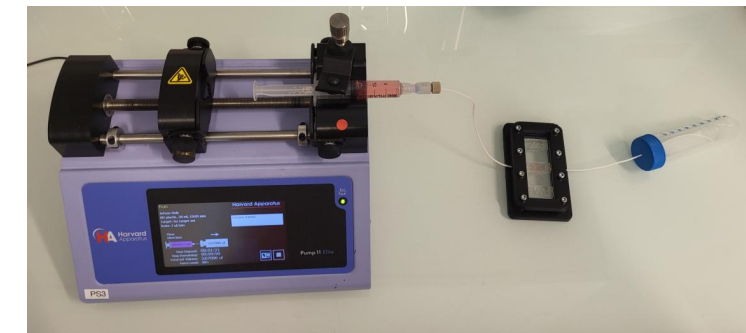
Medium perfusion in the channel for microvascularization formation
