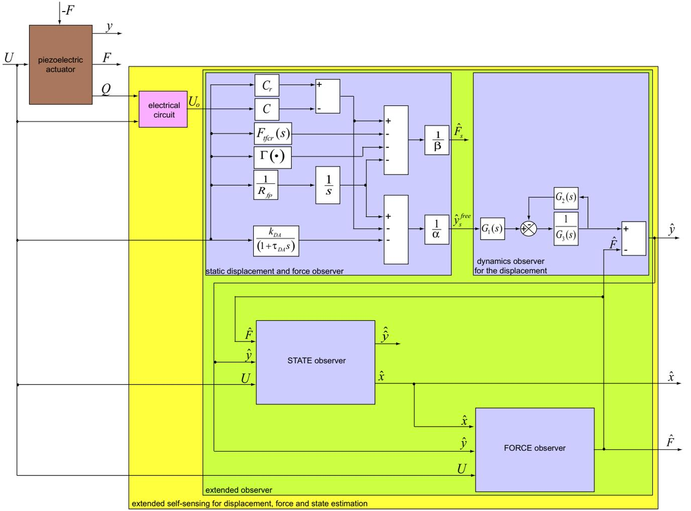
Fig. 4. Principle scheme of the extended complete self-sensing.
