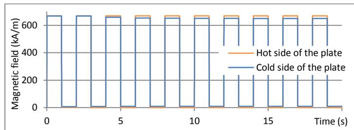
Fig. 5. Magnetic field in the gadolinium over time
