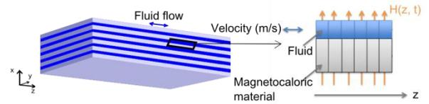
Fig. 2. 1D model for the thermal model
