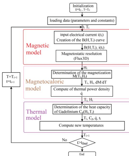
Fig. 3. Resolution algorithm of the model
