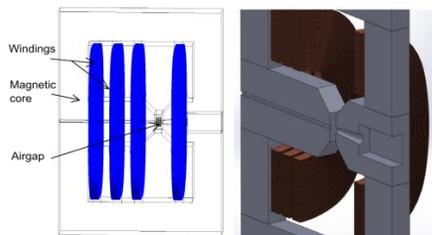
Fig. 4. 3D model of a special electromagnet
