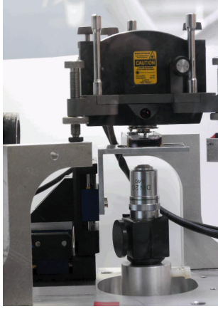
Fig. 10. AFM with substrate in liquid medium.
