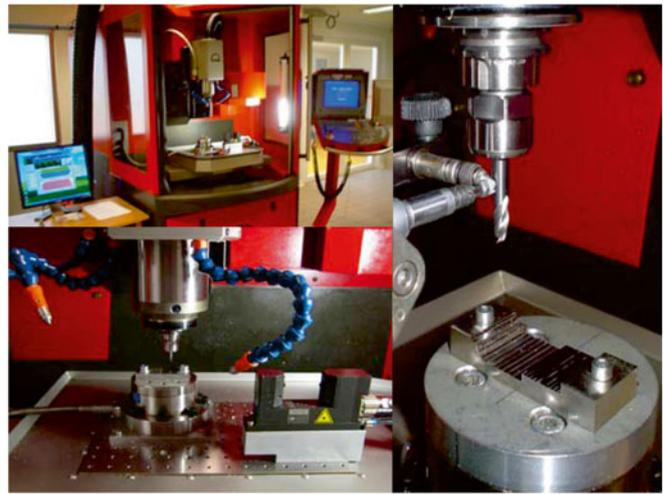
**Fig. 1** Assembly of the samples used for the experiments and pictures of the milling acquisition systems
