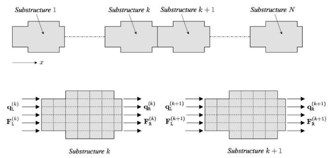
**Fig. 1** An illustration of a periodic waveguide [17].
