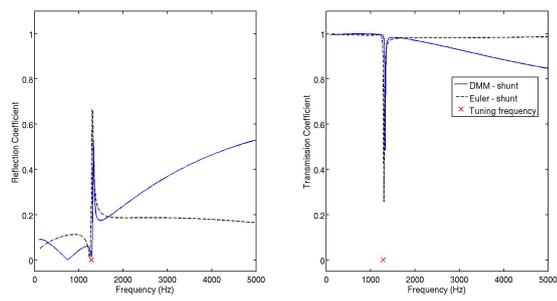
**Fig. 8** Comparison of reflection and transmission coefficients of the flexural mode in  $Z$ -axis between the results of the homogenized Euler-Bernoulli beam model and those of the DMM approach in case A. (Solid line)DMM results (Dashed line)Homogenized model results.
