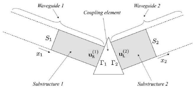
**Fig. 2** An illustration of the coupling between two different periodic waveguides [17].
