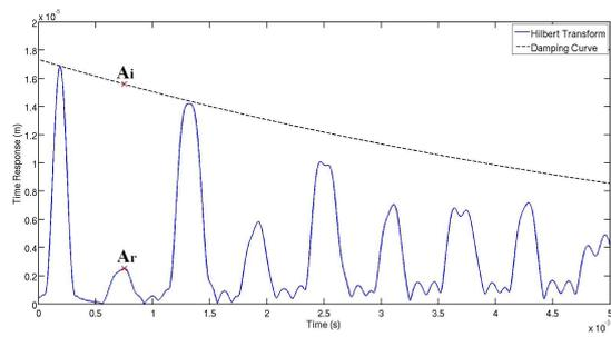
**Fig. 21** Hilbert Transform of the time response and the damping curve to extract the reflection coefficient of the tension/compression wave. (Solid line) Absolute value of the Hilbert Transform of the time response. (Dashed line) Damping curve based on spatial damping.
