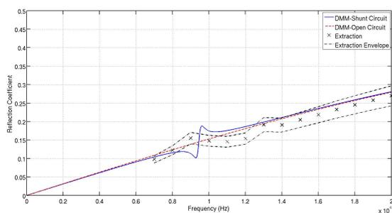
**Fig. 22** Comparison of reflection coefficients of the tension/compression wave in  $X$ -axis calculated through the DMM approach and the extraction procedure. (Solid line) Calculation with DMM, piezoelectric patch with shunt circuit. (Dashed line) Calculation with DMM, piezoelectric patch without shunt circuit. ( $\times$  markers) Calculation with extraction procedure. (Dash-dotted line) Envelope of the extracted reflection coefficients.
