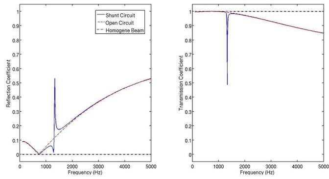
**Fig. 6** Reflection and transmission coefficients of the Z-axis flexural wave mode propagating in the beam in case A. (Solid line)With R-L shunt circuit (Dashed line)Open circuit (Dash-dotted line)Beam without piezopatches.
