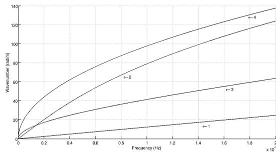
**Fig. 10** Dispersion curves of the wave modes propagating in the beam in case B and case C: (1) Tension/compression mode in  $X$ -axis (2) Torsional wave in  $X$ -axis (3) Flexural wave in  $Y$ -axis (4) Flexural wave in  $Z$ -axis. These wave modes are identified through their mode shapes (eigenvectors) issued from the WFE approach.
