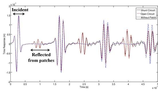
**Fig. 20** Time response of the structure under wave packet excitation. (Solid line) Piezoelectric patch with shunt circuit. (Dashed line) Piezoelectric patches without shunt circuit. (Dash-dotted line) Beam without piezoelectric patches.
