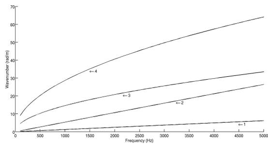
**Fig. 5** Dispersion curves of the wave modes propagating in the beam in case A: (1)Tension/compression wave in  $X$ -axis (2)Torsional wave in  $X$ -axis (3)Flexural wave in  $Y$ -axis (4)Flexural wave in  $Z$ -axis. These wave modes are identified through their mode shapes (eigenvectors) issued from the WFE approach.
