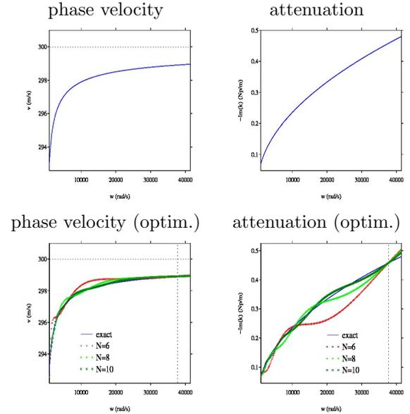
Fig. B.1. Dispersion curves in the linear regime ( $b = 0$ ), with  $c = 300$  m/s,  $\varepsilon = 1$  and  $\alpha = 1/2$ . Comparison between the original model (top) with fractional derivatives (1) and the diffusive representation model (6) where the coefficients are determined by optimization (bottom). The horizontal dotted line denotes  $c$ . The vertical dotted lines denote the range of optimization  $[\omega_{\min}, \omega_{\max}]$ .
