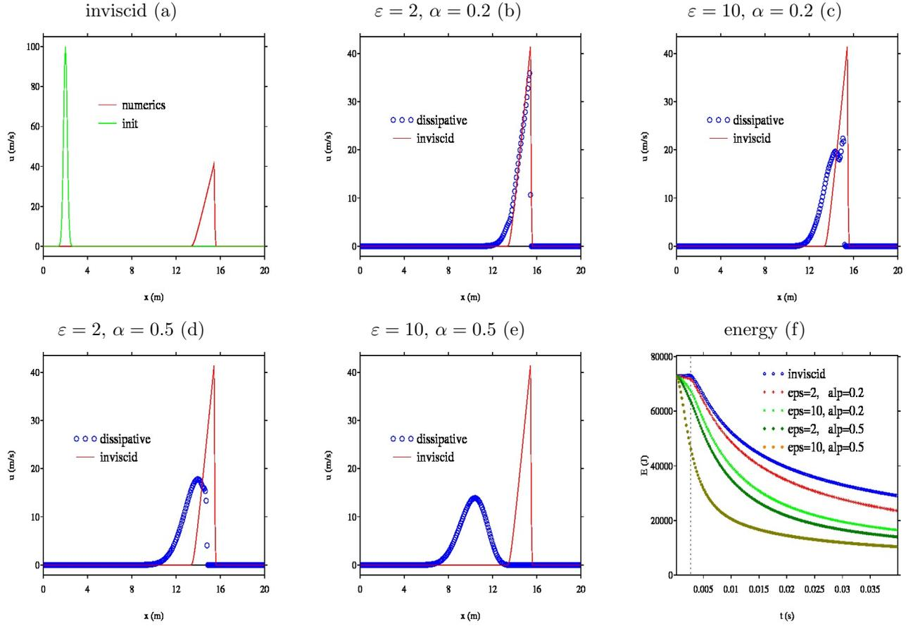
Fig. 1. Gaussian pulse. Snapshots of  $u$  in the inviscid case and for various dissipative parameters  $\varepsilon$  and  $\alpha$  (a-e). The subfigure (f) shows the time evolution of the energy; the vertical dotted line denotes the time of break  $t^*$  (18).
