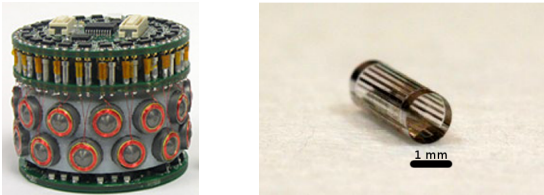
Fig. 1: Claytronics catom prototypes (left one with magnetic actuation, right one with electro-static actuation)
