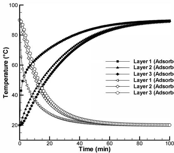
Figure 8. Temperature variation for the two adsorbers with time; layer 1:  $r = 20.2$  mm; layer 2:  $r = 29.8$  mm; layer 3:  $r = 39.8$  mm ( $R = 50$  mm;  $T_{\text{heat}} = 90$  °C).
