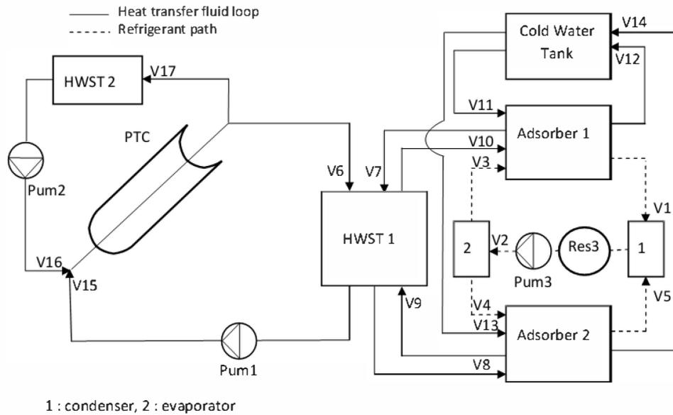
Figure 3. Schematic diagram of the solar powered continuous adsorption refrigeration system.
