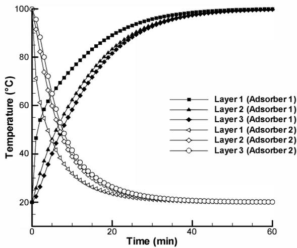
Figure 5. Temperature variation for the two adsorbers with time; layer 1:  $r = 20.2$  mm; layer 2:  $r = 29.8$  mm; layer 3:  $r = 39.8$  mm ( $R = 40$  mm);  $T_{\text{heat}} = 100$  °C).
