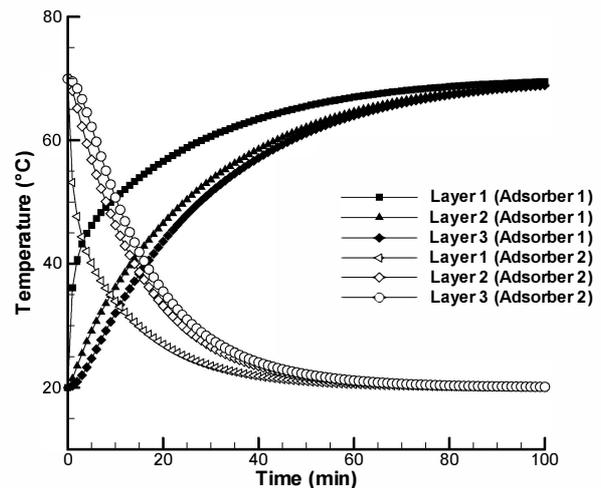
Figure 9. Temperature variation for the two adsorbers with time; layer 1:  $r = 20.2$  mm; layer 2:  $r = 29.8$  mm; layer 3:  $r = 39.8$  mm ( $R = 50$  mm;  $T_{\text{heat}} = 70$  °C).
