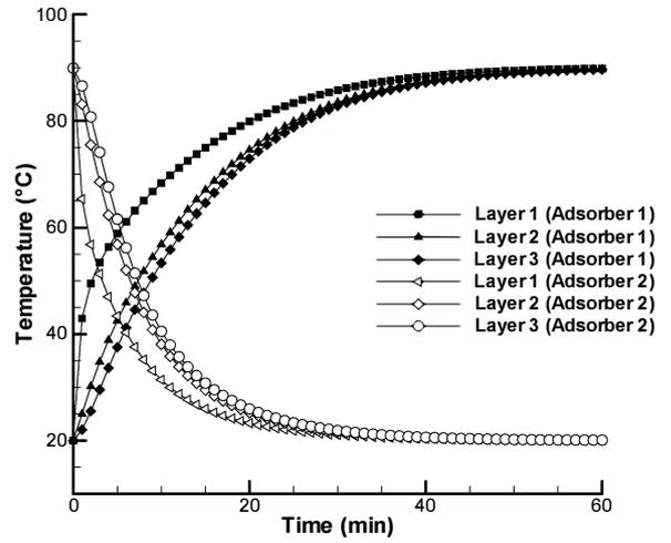
Figure 6. Temperature variation for the two adsorbers with time; Layer 1:  $r = 20.2$  mm; Layer 2:  $r = 29.8$  mm; Layer 3:  $r = 39.8$  mm ( $R = 40$  mm);  $T_{\text{heat}} = 90$  °C).
