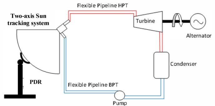
Figure 2. System of production of the electric energy.
