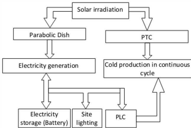
Figure 1. Schematic diagram of the global system.
