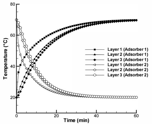
Figure 7. Temperature variation for the two adsorbers with time; layer 1:  $r = 20.2$  mm; layer 2:  $r = 29.8$  mm; layer 3:  $r = 39.8$  mm ( $R = 40$  mm);  $T_{\text{heat}} = 70$  °C).
