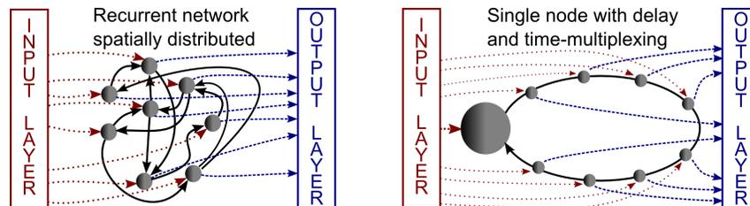
Fig. 1. (Left) Sketch of a traditional RC setup. (Right) RC based on a single nonlinear element subject to delayed feedback.
