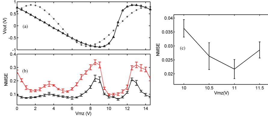
Fig. 4. (a) Experimentally recorded nonlinearity (dotted line) and operating point (solid line with triangles) as a function of the Mach-Zehnder bias voltage (offset phase). (b) Test prediction error (NMSE) for the Santa Fe time-series prediction task with 400 virtual nodes for two-valued (dashed line) and six-valued (solid line) input masks. (c) NMSE of the predicted time-series for an improved detection with 5:1 oversampling and six-valued mask.
