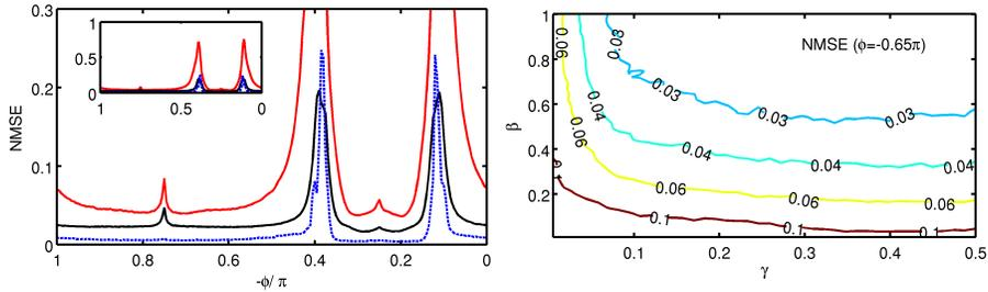
Fig. 2. (Left) NMSE test prediction error in the Santa-Fe time series prediction for  $\beta = 0.8$  and  $\gamma = 0.45$  as a function of the offset phase  $\Phi$ . Red (blue) line corresponds to a binary mask in the presence (absence) of quantization noise. Black line corresponds to a six-valued mask in the presence of quantization noise. (Right) Colour-coded NMSE prediction error in the  $\beta - \gamma$  plane for  $\Phi = -0.65\pi$  and a six-valued input mask.
