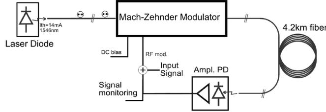
Fig. 3. Experimental implementation of the optoelectronic oscillator with delay.
