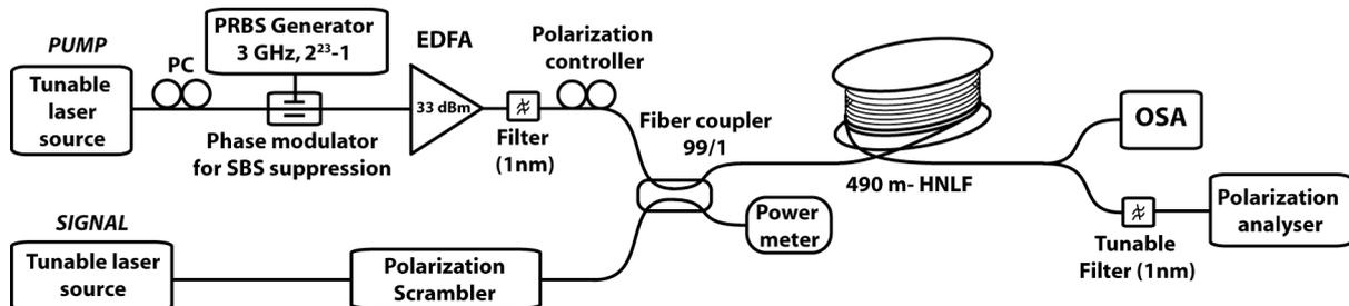
Fig 1. Experimental arrangement of the fiber-optical parametric polarizer. EDFA : Erbium-doped fiber amplifier. OSA : Optical spectrum analyzer. PRBS : pseudorandom bit sequence. PC : Polarization controller.
