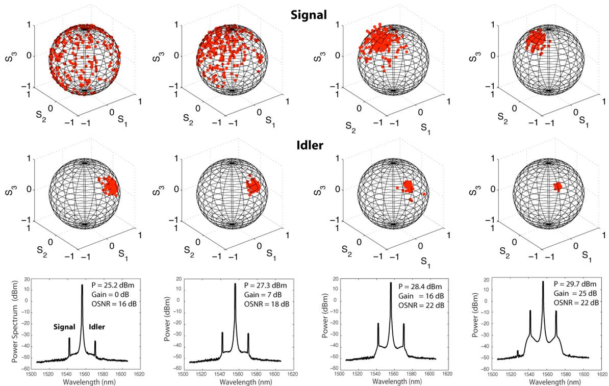
**Fig. 2.** Output state of polarization (SOP) of the signal (top) and idler (middle) waves measured by a polarimeter and visualized on the Poincaré sphere of unit radius, while input signal SOP is scrambled and pump power increases from 25.2 dBm to 29.7 dBm. Bottom: corresponding output gain spectra. The input pump power is indicated in insets together with the on/off gain and the signal OSNR.
