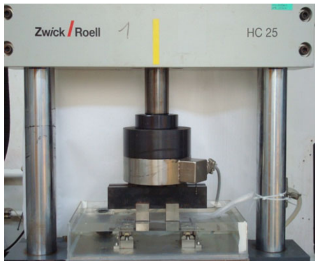
Fig. 2 Fatigue test set-up in four-point bending in natural circulating sea water
