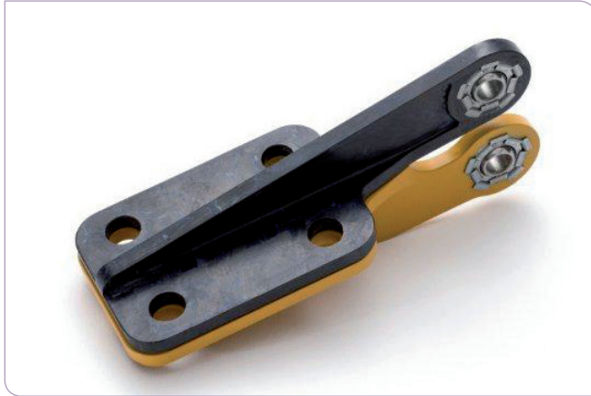
Fig. 2: TP-CFRP door hinge and original CNC-machined steel hinge [courtesy of Eurocopter Germany GmbH]
