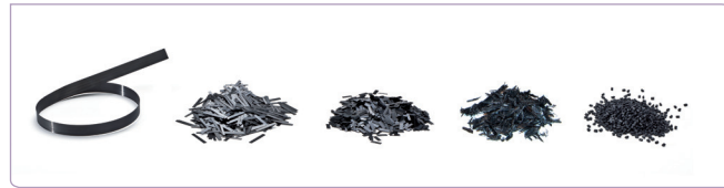
Fig. 6: From left to right, UD tape, 20mm chopped tapes, 10mm chopped tapes, recycled fragments, injection moulding granules
