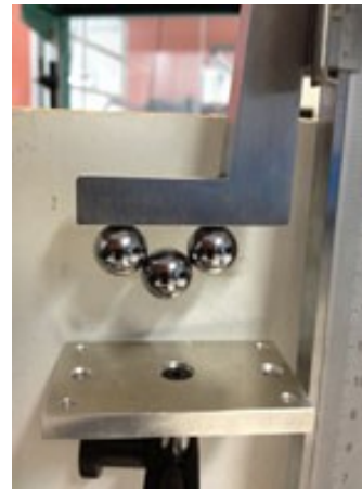
Figure 6: The 3 magnets in position «loop».
